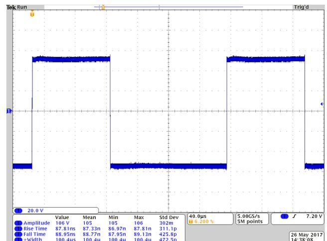
+50 V & -50 V, 4 kHz, 100.4  $\mu$ s, 344 pF Load
