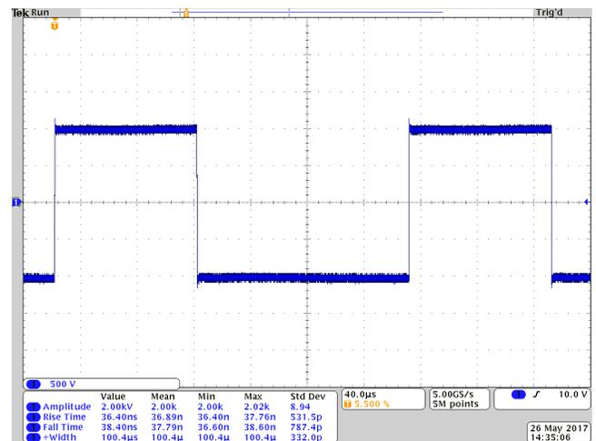
+1000 V & -1000 V, 4 kHz, 100.4  $\mu$ s, 344 pF Load
