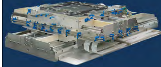
Figure 2. A motion amplified, flexure-guided actuator based on a multilayer piezo stack. Piezo flexure drives can last 100 billion cycles!
