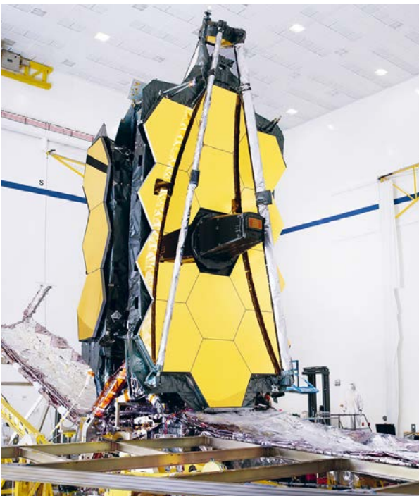
Folding and packing the Webb before launch (© ESA).
