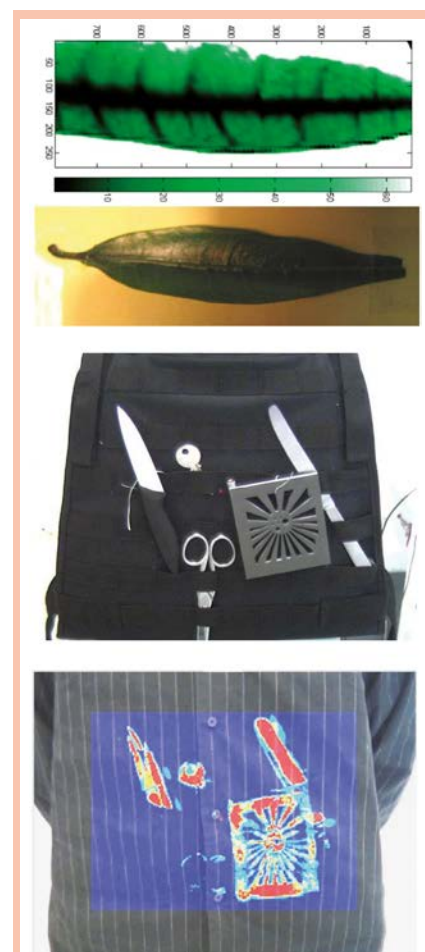
Figure 1. Examples of THz images (taken with CEA-Leti sensors). (a) Leaf in transmission. (b) Visible image of objects concealed on the chest. (c) Raw THz image of objects concealed under a shirt.
