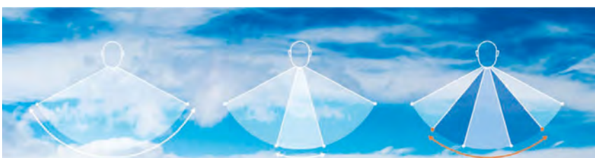
Figure 7: FOV in AR glasses with different indices. Left: FOV with binocular vision. Centre: FOV with display glass, n = 1.5 . Right: FOV for AR glass with n = 1.6 (smallest FOV) up to n = 2 (largest FOV). Taken with permission from [6].
