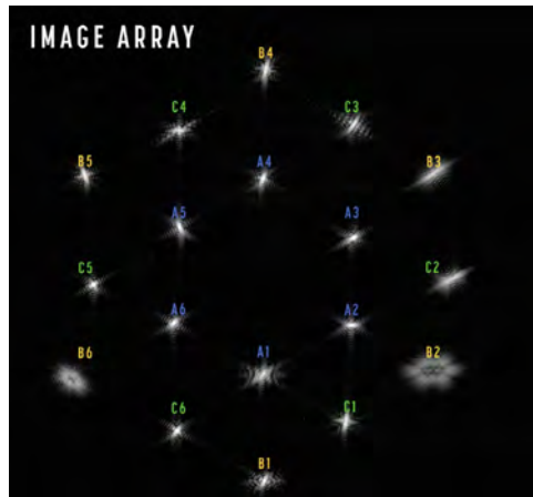
Figure 1: Diffraction image of the same star by each of the 18 segments of the primary mirror. The segments are tilted to create a hexagonal grid on the NIRCcam instrument. Each image is labelled with the corresponding mirror segment that captured it. Credits: NASA/STScI/J. DePasquale. https://blogs.nasa.gov/webb/2022/02/18/webb-team-brings-18-dots-of-starlight-into-hexagonal-formation/
