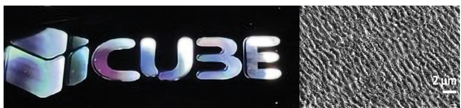
Figure 3. (left) color effect by surface texturing achieved by (right) Laser Induced Periodic Structures (LIPSS) at smaller scale (zoom).
