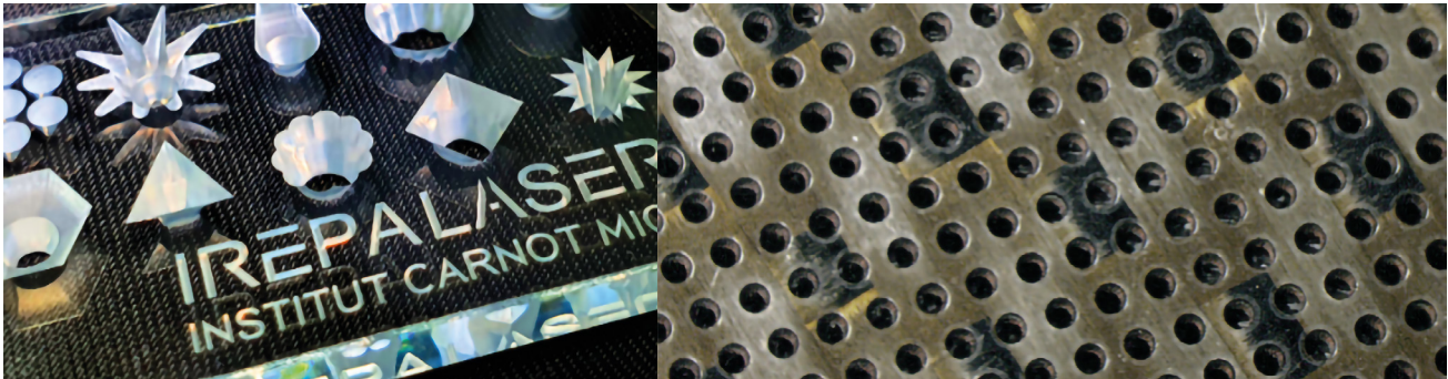
Figure 4. 3D glass manufacturing and micro-drilling in stainless steel plate by IREPA LASER using USP laser.
