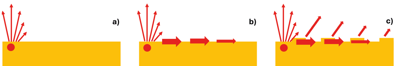
Figure 3. Sketch of the mechanism producing spatial coherence and directional emission. a) Thermal emission by a hot body. Each volume element (red disk) contains charges with random thermal motion. The corresponding current density emits light which is transmitted by the interface (red arrows). b) Thermal emission by a hot body sustaining a surface wave. In addition to the transmitted light, a surface wave (thick horizontal line) is excited. The dispersion relation of the surface wave is denoted k_{sw}(\omega) . The surface wave propagates along the interface and decays exponentially due to the losses in the material. As a consequence, the field is correlated over a distance limited by the surface wave decay length. c) Coherent thermal emission. When a grating with period d is ruled on the interface, the surface wave is diffracted in a direction \theta given by the grating law \omega/c \sin \theta = k_{sw}(\omega) - 2\pi/d .
