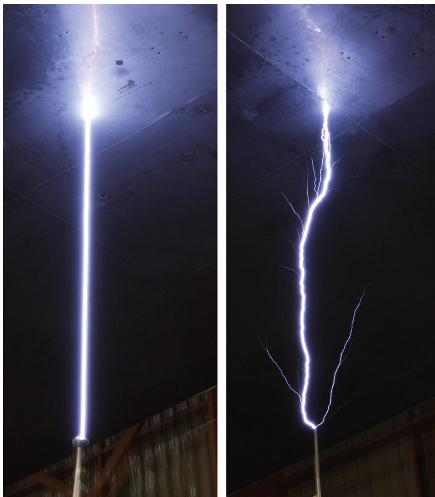
Figure 1. Photograph of a 2 m-long electric discharge guided by laser filamentation (left) and without laser filament (right).
